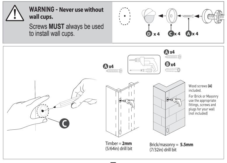
9. Reinstall gate inserting bolts with rubber pads into Wall Cups (C).
