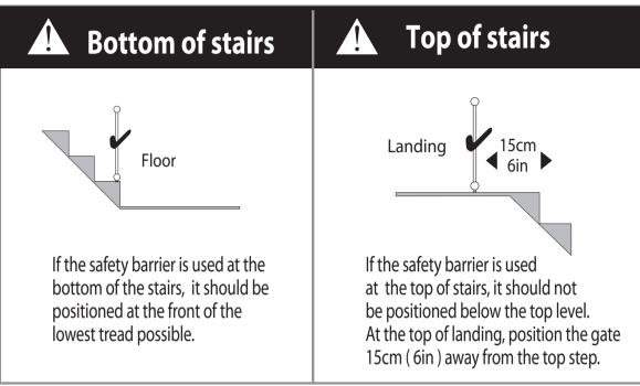
**CAUTION:** With any pressure mounted gate, a construction bar is required across the base.
