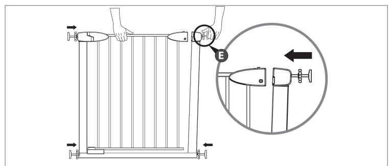
4. Place the gate in the opening so that the bottom of the Gate Frame is completely flat on the floor, and it is perpendicular to the opening and the floor.
