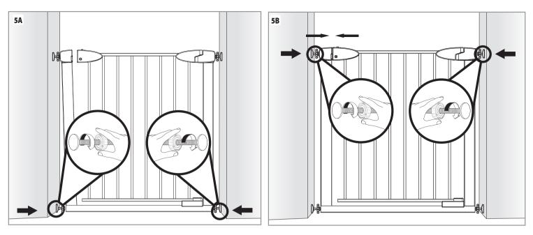
When correctly tightened, the distances between Tension Knobs and Rubber Pads should be equal.
