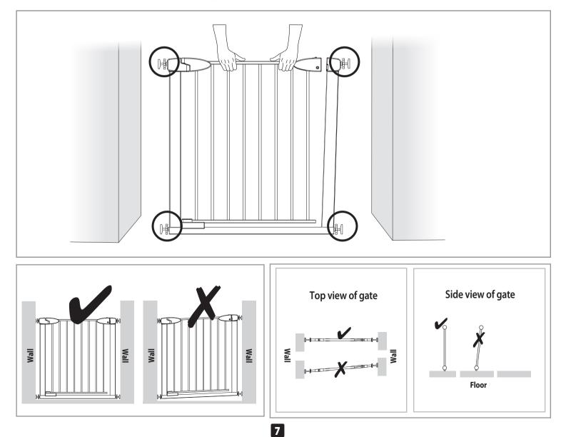
5. Tighten both of the lower Tension Knobs (E) by turning them at the same time. NOTE: Make sure the bottom of the gate frame remains completely flat on the floor. Next, tighten both of the upper Tension Knobs (E) by turning them at the same time.
