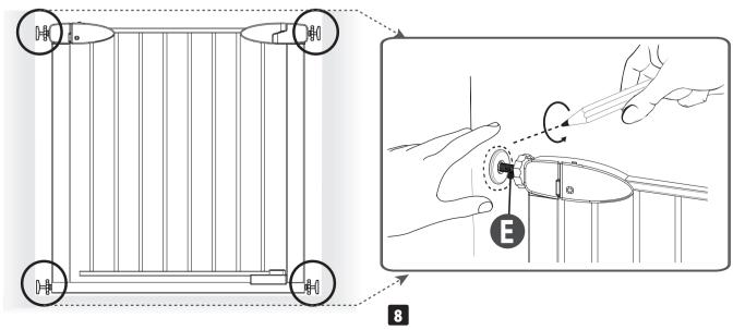
7. Loosen the Tension Knobs and remove gate. Line up Wall cups with marks on wall.
